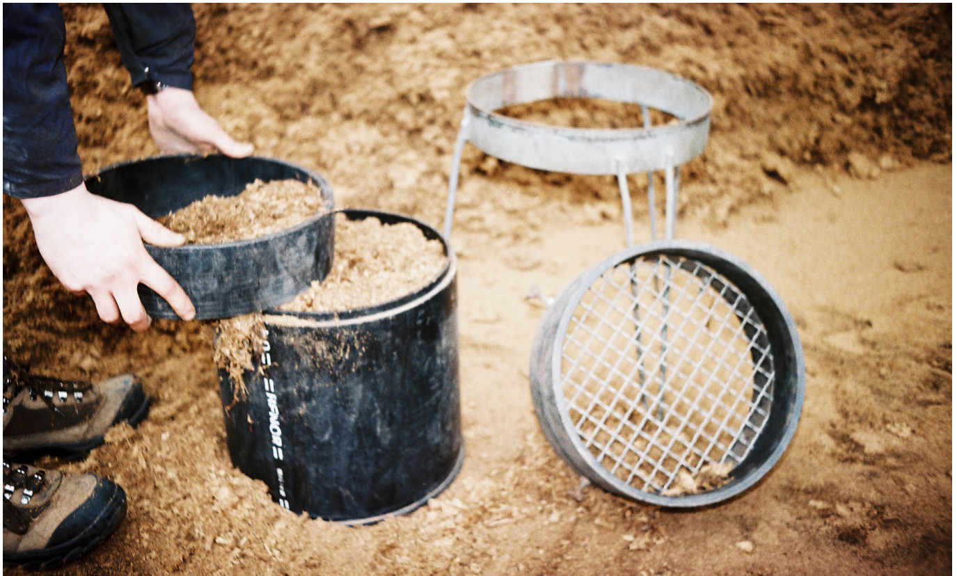
The manual way of determining the bulk density according to the EN12580.
